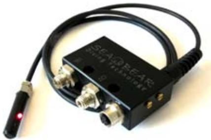
condensation on the front lens during cold water diving. The electronic compartment was encapsulated in black polyurethane.
