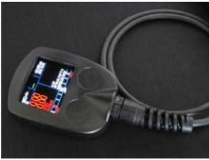
external electrical interferences are reduced. Therefore, it was convenient to use an interface based on ground referenced single-ended voltage inputs, rather than a differential pair of CAN.
